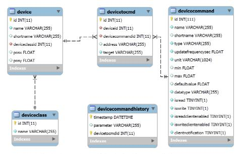
*Figure 2* Basic database schema of the device hierarchy within the LISI Core framework
