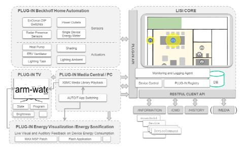
*Figure 1* LISI Core – System architecture and various plug-ins (as used in the Solar Decathlon Team Austrias LISI smart home)
